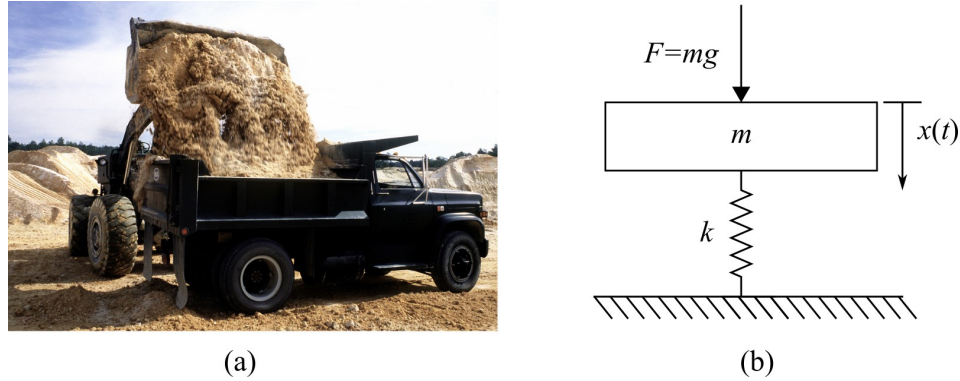
Figure 4.8: Dump truck being loaded with dirt showing (a) dirt going into the truck bed a ; and (b) the single-degree-of-freedom vibration model.
