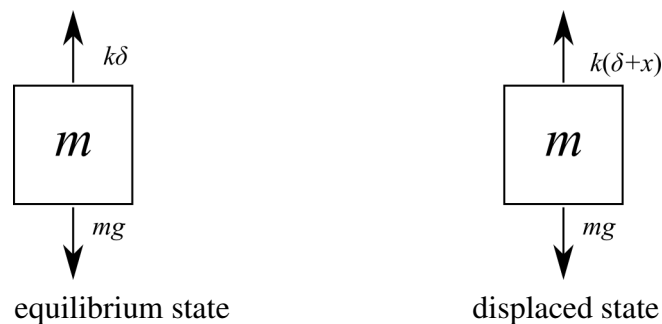
Figure 1.19: Equivalent forces for a 1 DOF spring-mass system with movement in the vertical direction
