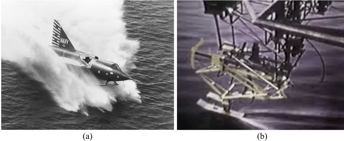
Figure 3.26: The Convair F2Y Sea Dart, showing: a) XF2Y-1 Sea Dart (BuNo 135762) during landing. This airframe disintegrated in mid-air over San Diego Bay, California (USA) during a demonstration flight on November 4th, 1954 killing test pilot Charles E. Richbourg after the airframe limitations were exceeded a , and b) the hydro-skis undergoing extensive testing on a pantograph mounted on a speed boat to study the forces transmitted to the airframe from the hydro-skis b .
